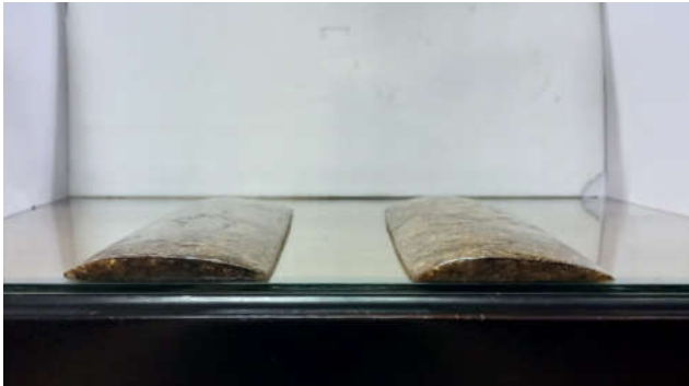
Fig. 10. Black Bamboo Composite SG6042 Wind Turbine Blade
