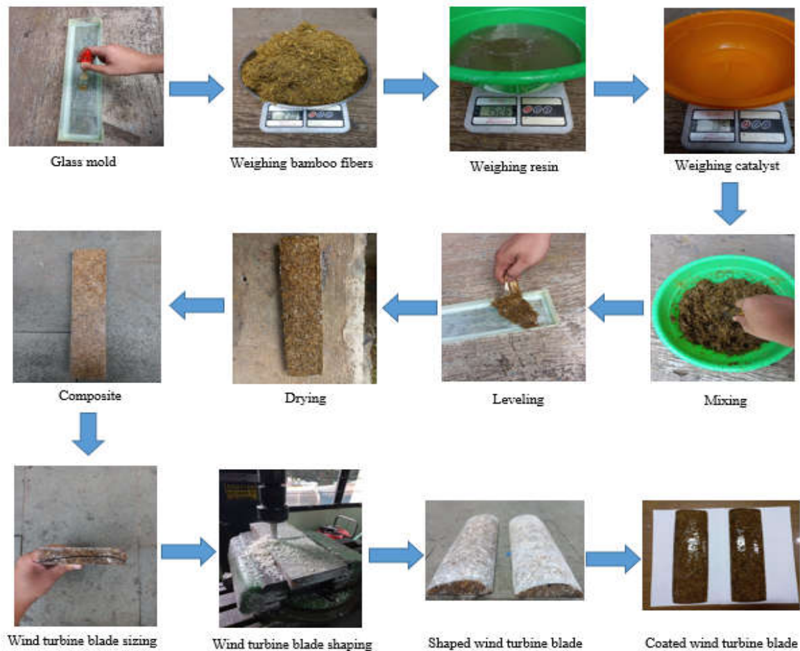
Fig. 8. Wind turbine blade manufacturing process.
